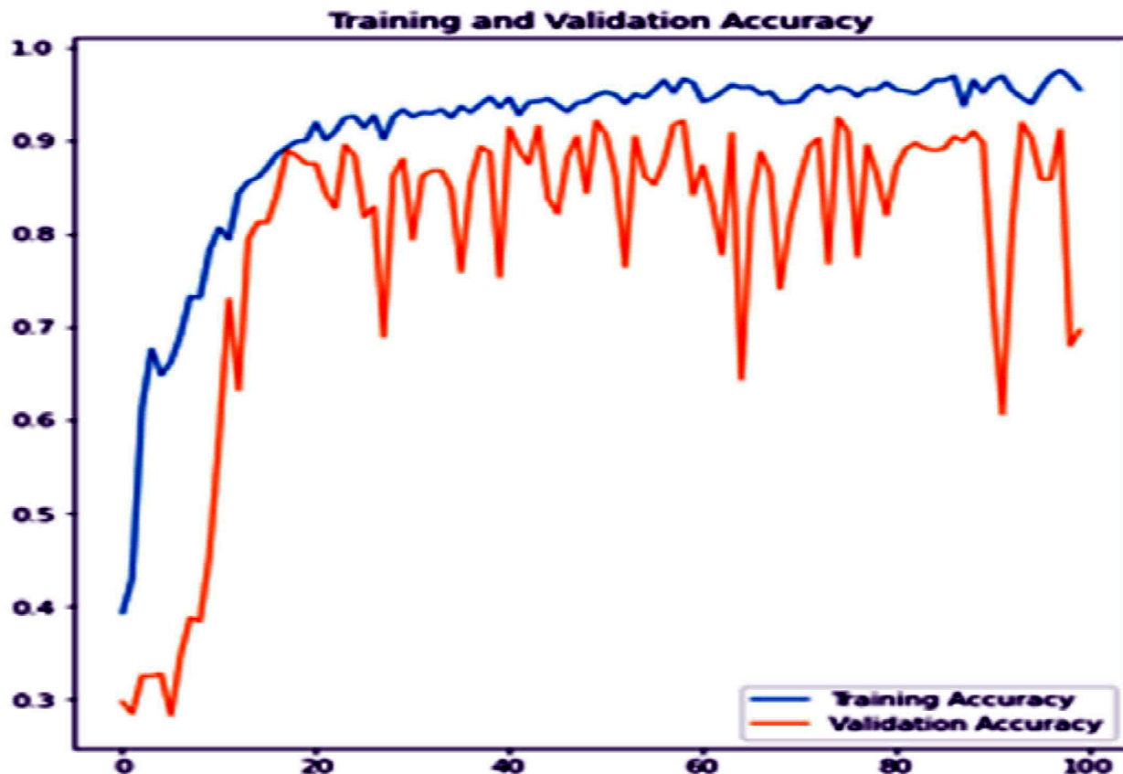
Fig. 6: Accuracy plots for training and validation of PDCNN
