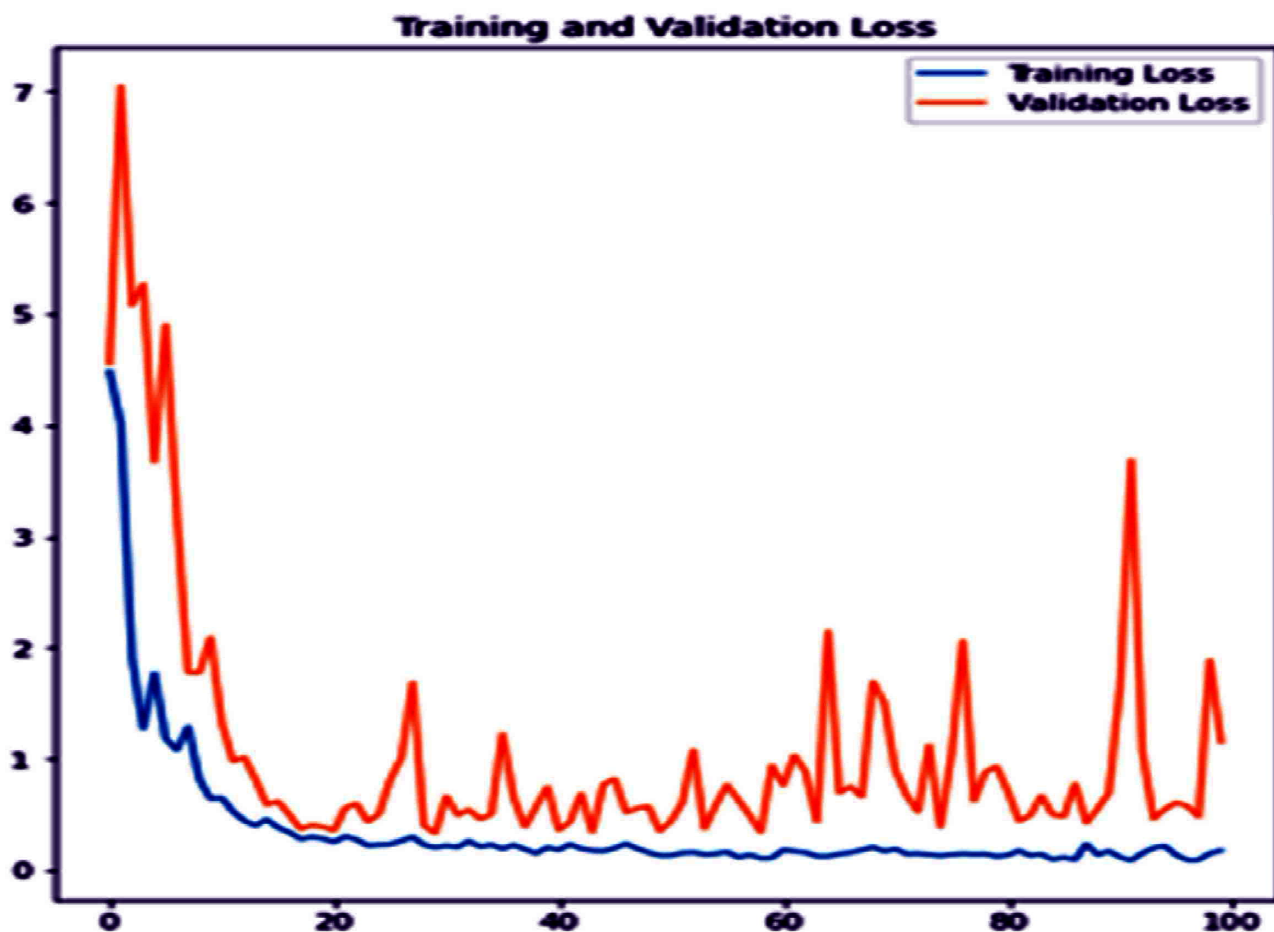
Fig. 7: Plots for validation and training loss of PDCNN
